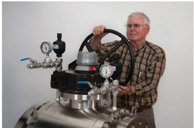
FIGURE 2. Verifying calibration and operation of a Trunnion-Mounted Ball Valve.
