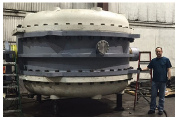
FIGURE 1. Shell test of a 126-inch Butterfly Valve
