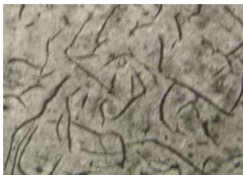
FIGURE 5. Ductile Iron at 400X
