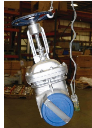
FIGURE 3. How NOT to lift a Gate Valve (Demonstration by United Valve)
