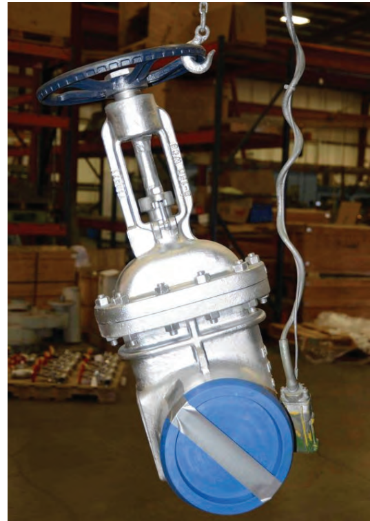
FIGURE 3. How NOT to lift a Gate Valve (Demonstration by United Valve)
