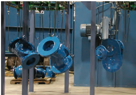
FIGURE 3. Conveyor System for Fusion Bonded Epoxy Process
