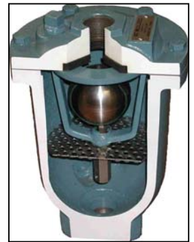
Well Service Air Valve High capacity exhaust and intake during turbine pump start up and start down.
