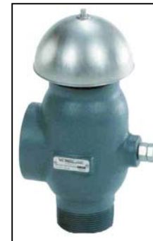
Dual-Port Throttling Device Controls the exhaust of air to control surges in the pump column and provides full air inflow through a hooded top port.
