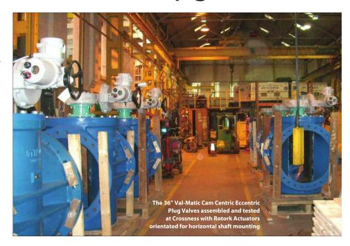
products' ability to be able to withstand harsh process environments, with its hard wearing and non-stick fusion bonded epoxy coating, coupled with a unique bearing arrangement and grit guards to extend longevity.
