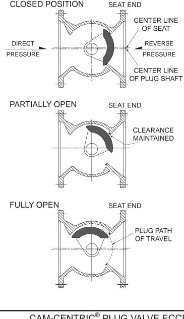
The eccentric action forces the resilient plug firmly against the seat, assuring a positive valve shut-off. An adjustable limit stop on the actuator allows the plug to be turned further into the seat, providing extended service life.
