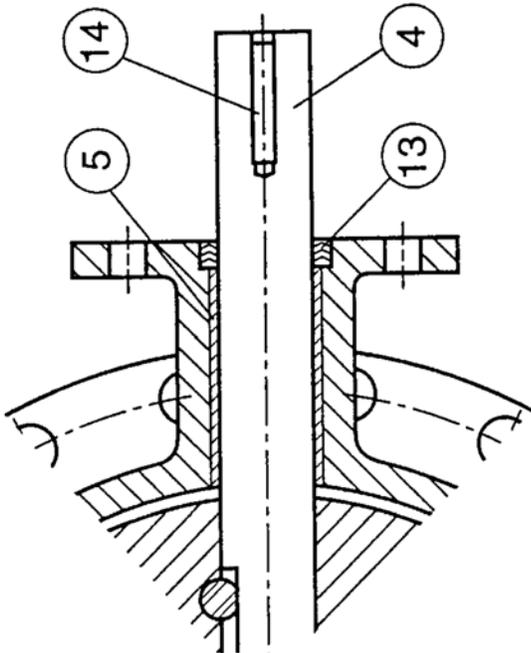
FIGURE 9. 3"-24" PACKING ASSEMBLY
