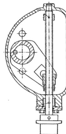
FIGURE 8. TRAVELING NUT ACTUATOR
