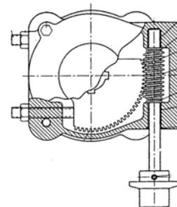
FIGURE 7. WORM GEAR ACTUATOR
