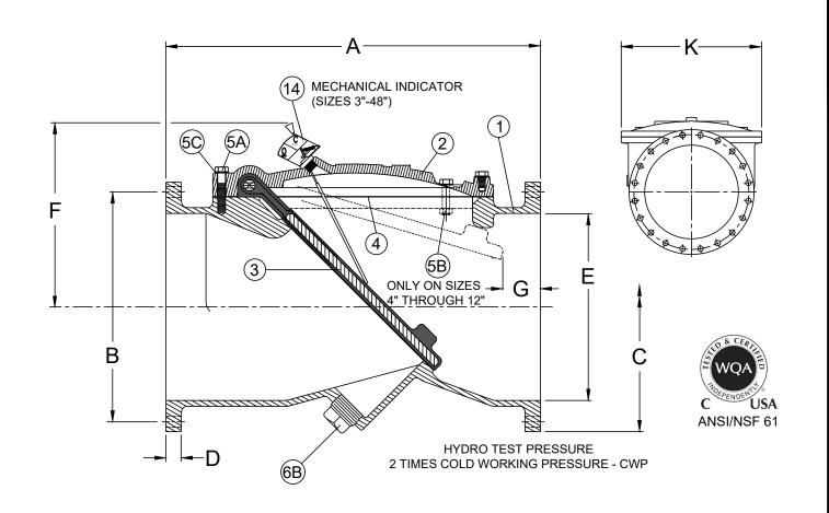
SEE DRAWING NO. VM-503AMI-M FOR STANDARD MATERIALS OF CONSTRUCTION
