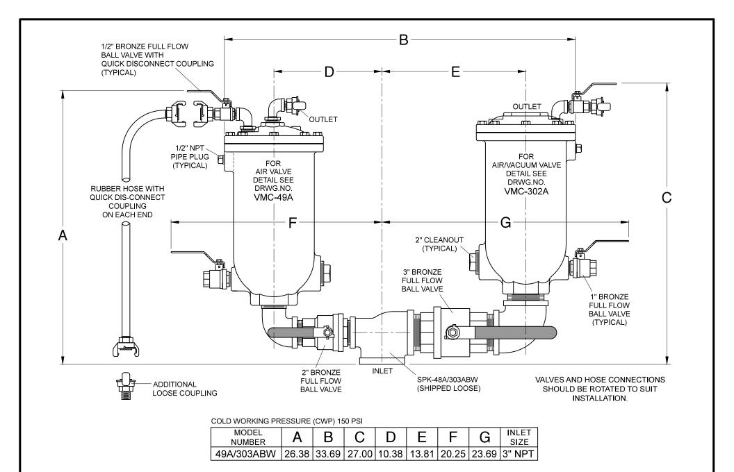
WASTEWATER COMBINATION AIR VALVE WITH BACKWASH ACCESSORIES
