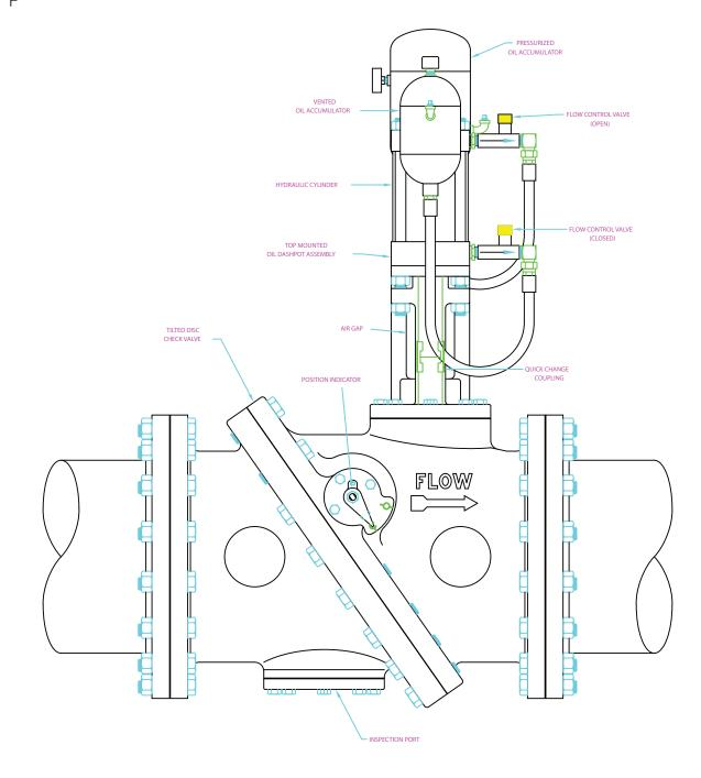
TILTED DISC CHECK VALVE DETAIL
