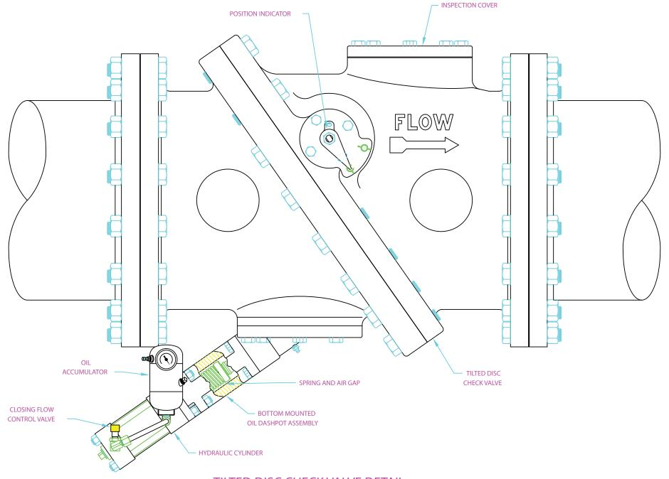
TILTED DISC CHECK VALVE DETAIL
