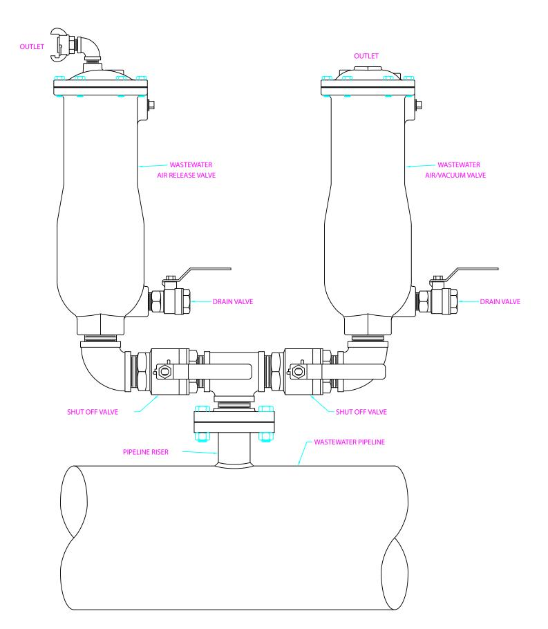
DUAL BODY COMBINATION AIR VALVE FOR WASTEWATER SERVICE
