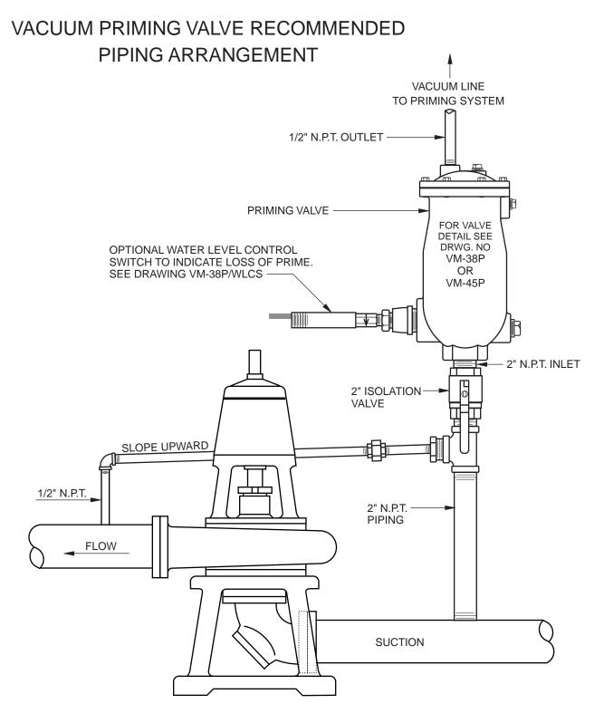
THE PURPOSE OF THE VACUUM PRIMING VALVE IS TO AUTOMATICALLY ALLOW AIR TO BE DRAWN OUT OF THE PUMPING SYSTEM UNTIL THE PUMP FILLS WITH WATER.
