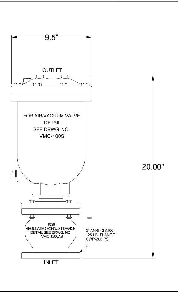
DATE 3" SURGE-SUPPRESSION AIR/VACUUM VALVE 1-27-17 DRWG. NO. AL VALVE AND MANUFACTURING CORP.
