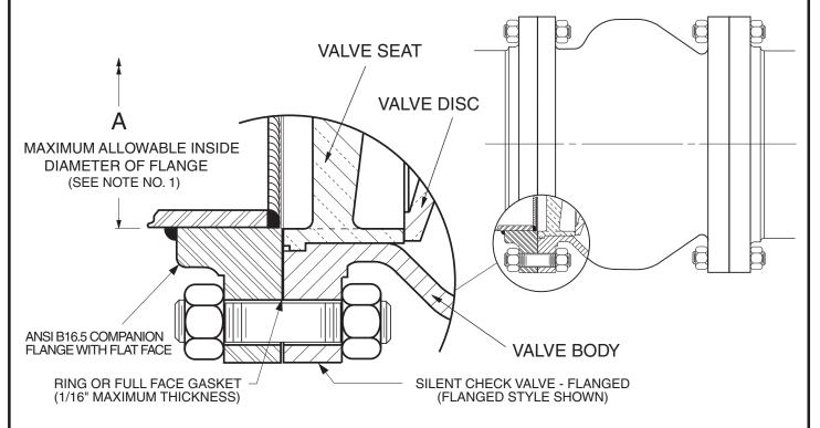
NOTE NO. 1 - THE MATING COMPANION FLANGE I.D. MUST OVERLAP THE VALVE SEAT. THIS IS REQUIRED TO PROVIDE PROPER SEAT RETENTION.
