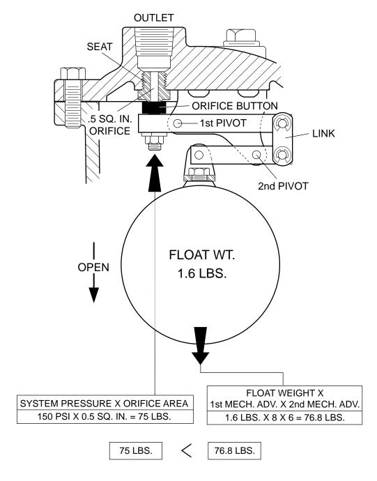
CONCLUSION: VALVE WILL OPEN AND VENT ACCUMULATED AIR.
