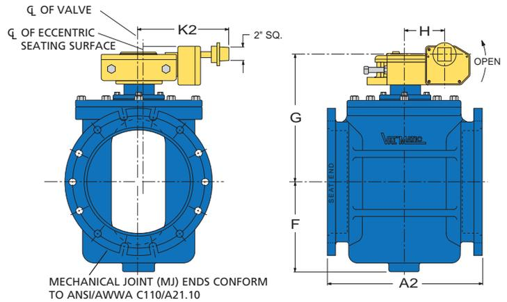
MECHANICAL JOINT (MJ) ENDS CONFORM TO ANSI/AWWA C110/A21.10
