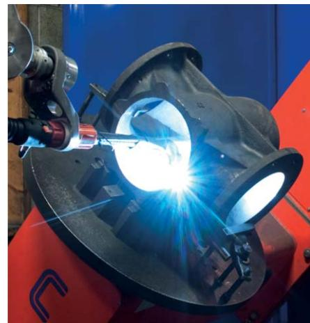
Figure 3. Robotic welding of nickel seat
