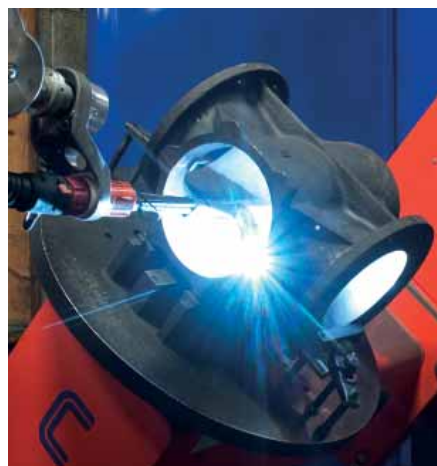
Figure 3. Robotic welding of nickel seat
