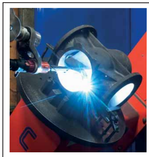
Figure 4. Robotic welding of nickel seat
