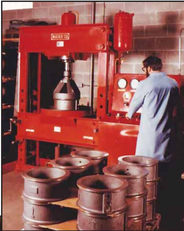
Dual Disc® Check Valve Hydrotesting
