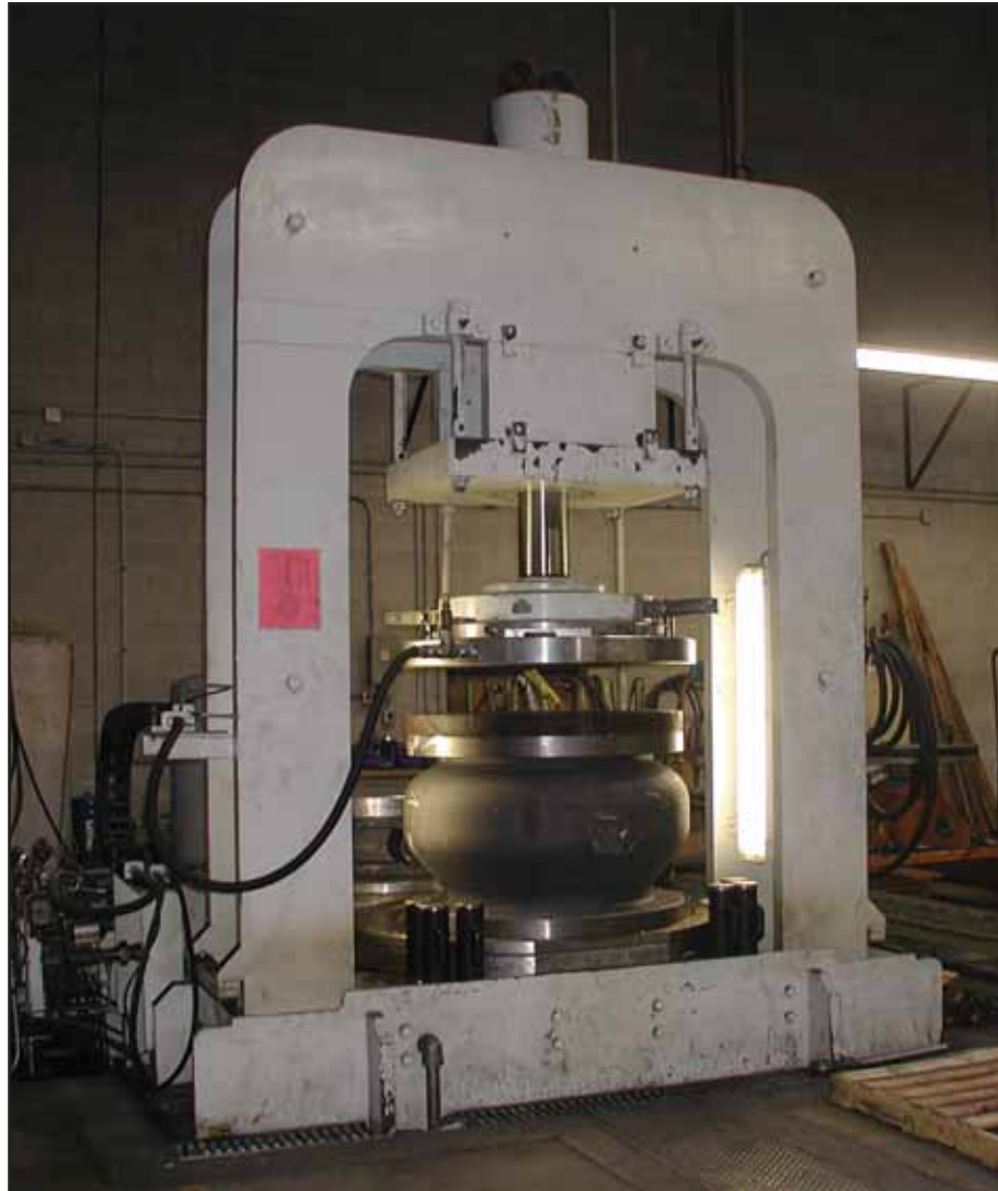
Silent Check Valve on a Test Stand
