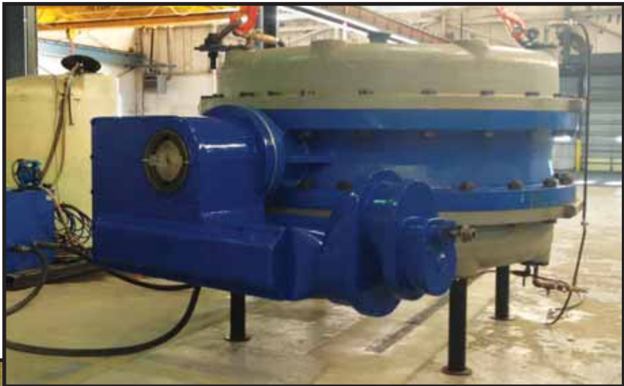
American-BFV® Butterfly Valve on Test Stand
