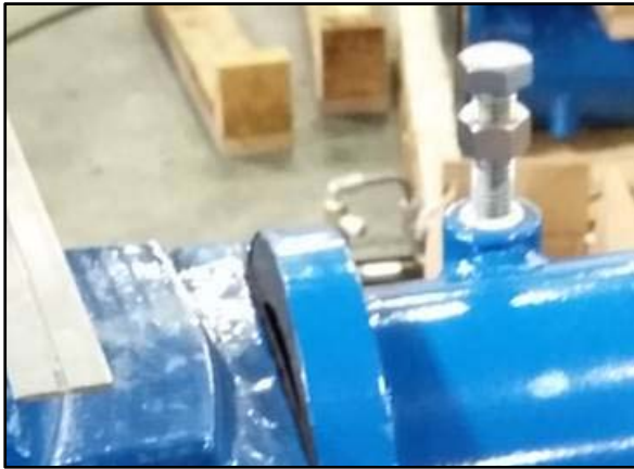
FIGURE 1. TYPICAL STOP BOLT
