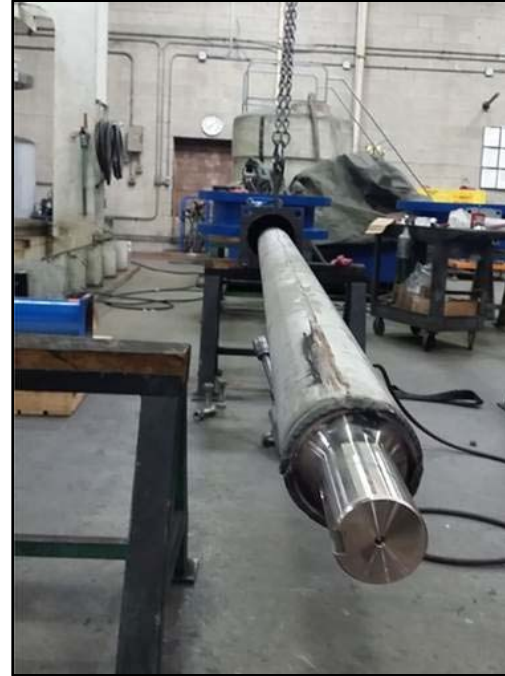
FIGURE 4. INSTALLING INNER SHAFT
