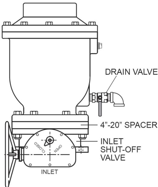
**Figure 3. Inspection Piping**
