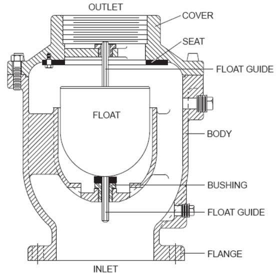
Figure 1. 4"-20" Air/Vacuum Valve
