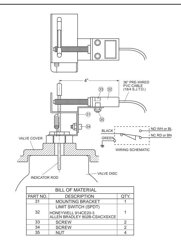
THE SWING-FLEX  $^{(8)}$  LIMIT SWITCH IS SCADA (SUPERVISORY CONTROL AND DATA ACQUISITION) COMPATIBLE FOR APPLICATIONS REQUIRING OPEN/CLOSE INDICATION.
