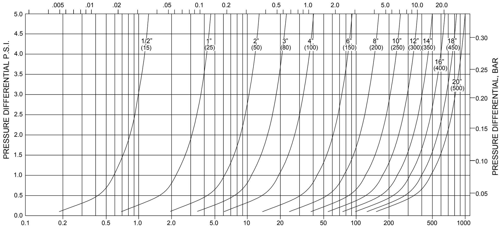
FLOW OF AIR THRU AN ORIFICE IN S.C.F.S.
