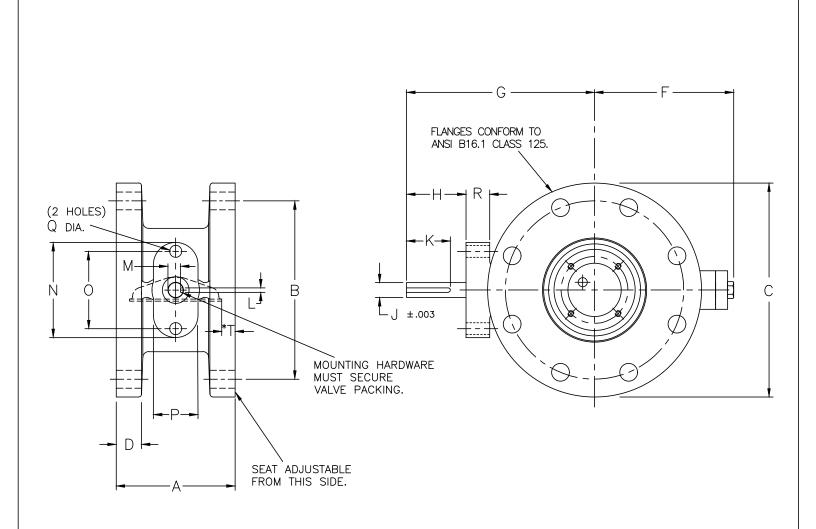
VALVE DRAWN TO SCALE. \*DISC SHOWN ROTATED 90°
