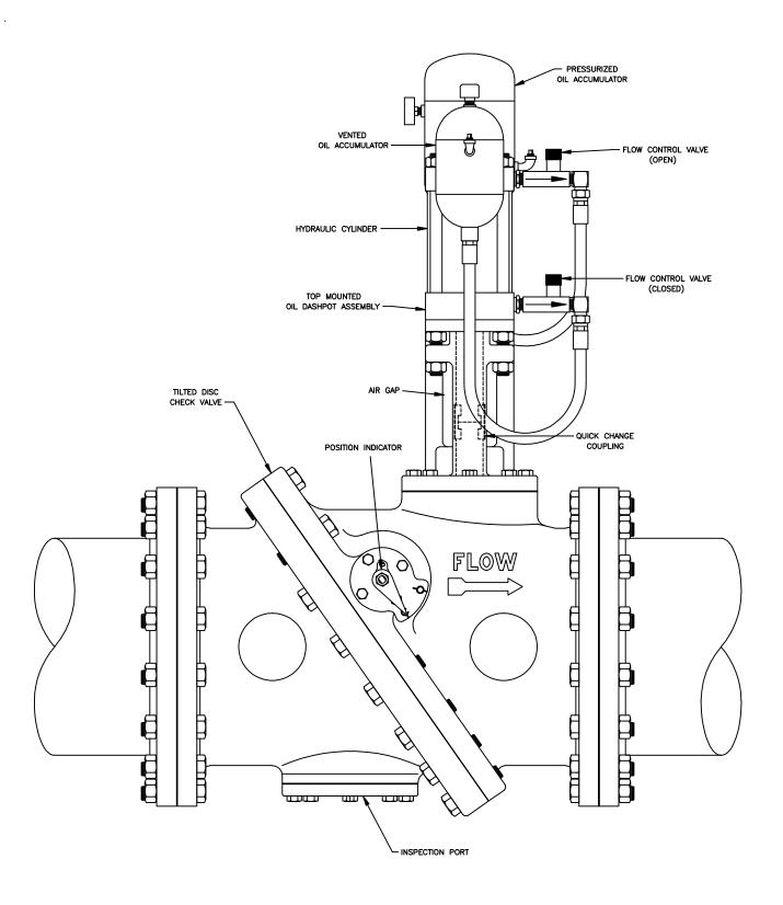
6"-54" TILTED DISC CHECK VALVE DETAIL
